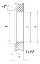
Installation direction: o-ring sits on chamfer.
